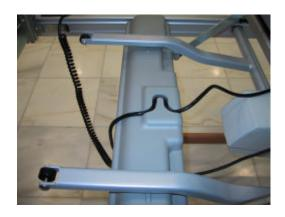
10. Reconnect all plugs to sockets on OKIMAT and replace the socket cap.
