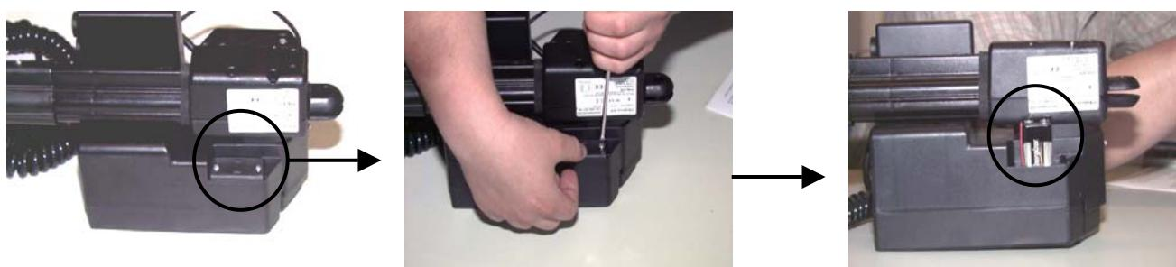
Fig. 25: exchanging the backup battery
