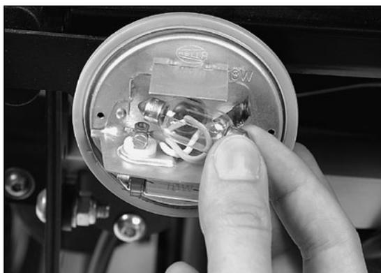
Fig. 44 Replacing the direction indicator bulb
