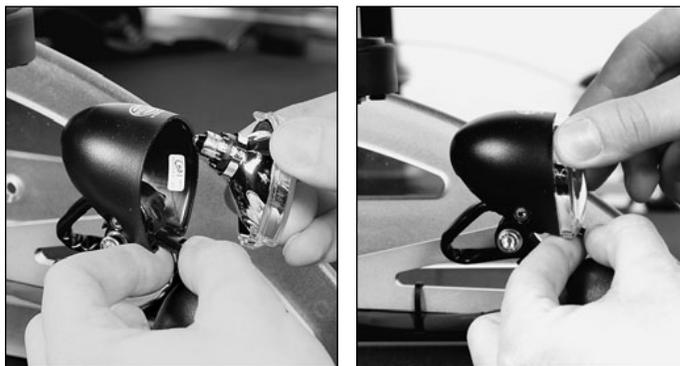
**Fig. 41** Replacing the front halogen lamp
