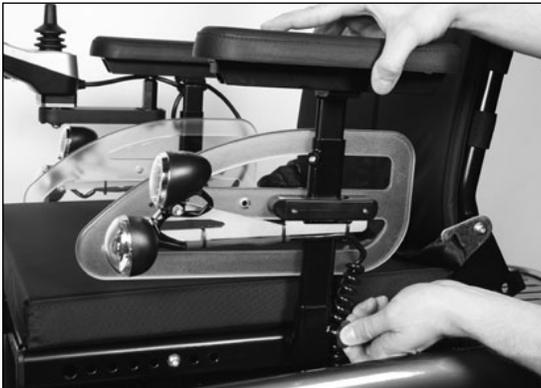
**Fig. 9** Loosening the thumb screw for removal of the side panel with armrest
