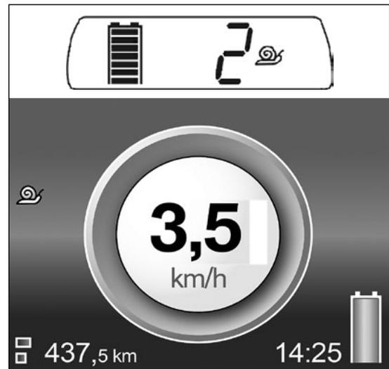
Fig. 23 Creep speed – Control panel display / LCD display
