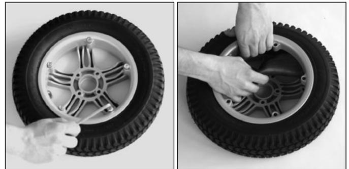
Fig. 40 Removing the casing
