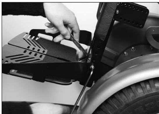
Fig. 13 Adapting the footrest(s) to the lower leg length
