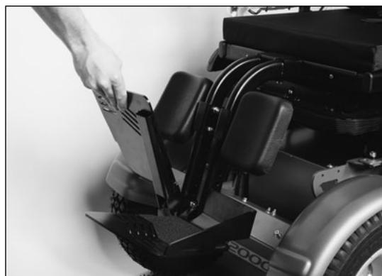
**Fig. 6** Folding the footplates up
