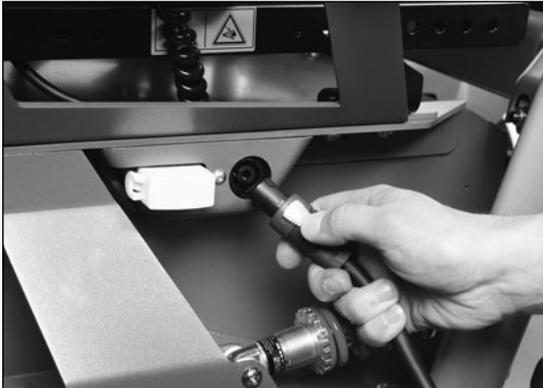
Fig. 22 Connecting the battery charger to the power wheelchair
