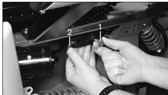
Fig. 21 Releasing the brake
