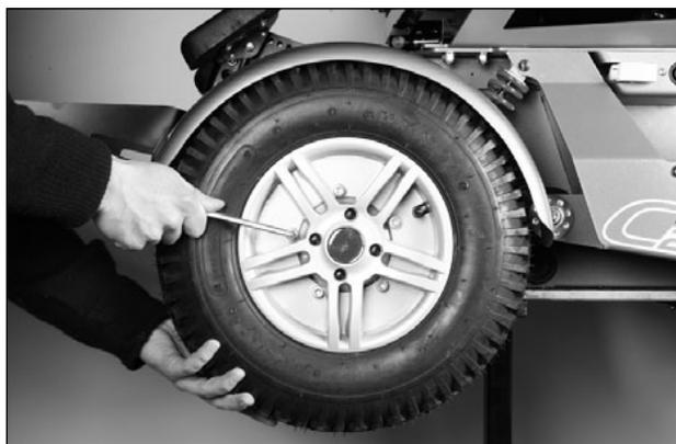
Fig. 39 Disassembling the drive wheel
