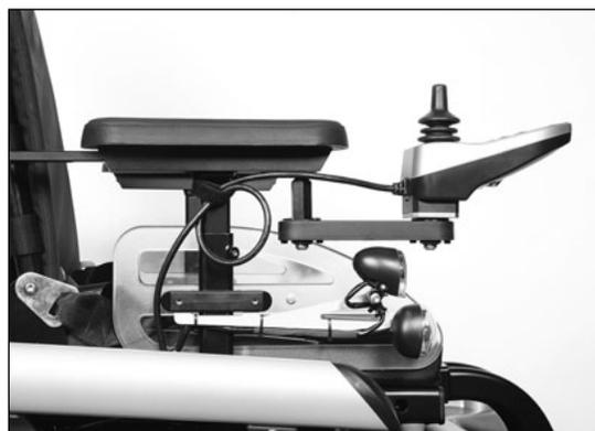
Fig. 30 Control panel holder, swing-away
