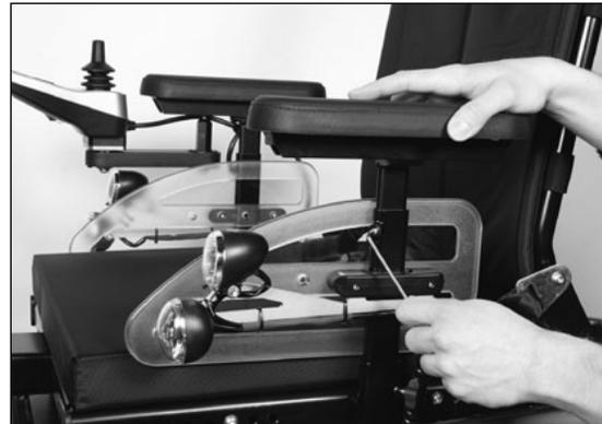
**Fig. 10** Adapting the armrest to the upper arm length
