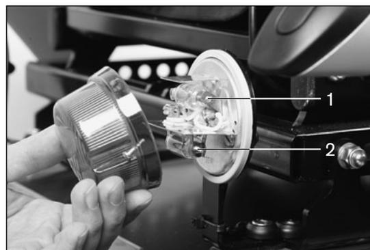
Fig. 43 Disassembling the rear lights
