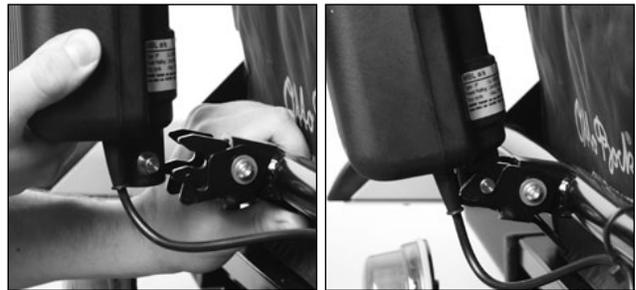
Fig. 4 Inserting the cross bolt into the holder; locked cross bolt
