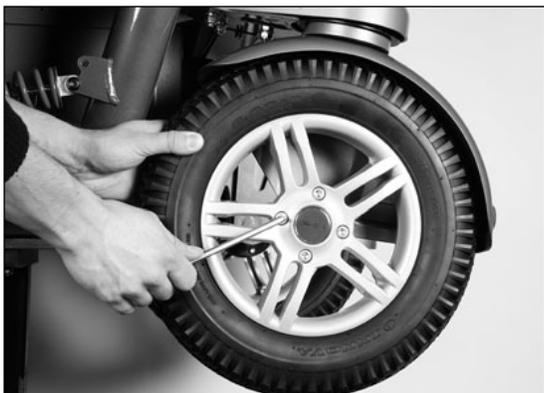
Fig. 38 Removing the caster wheel
