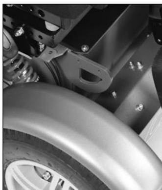
**Fig. 5** Eyebolts on the driving side
