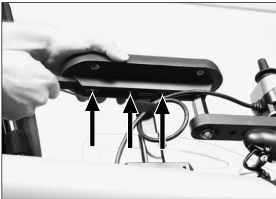
Fig. 12 Adapting the control panel
