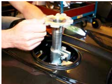
Adjust the seat post to the desired position. The seat post is marked with a ring at each centimeter.
