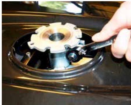
Loosen the counter nut. Use spanner, 17 mm.
