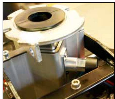
Release button pressed out. Now the seat tube can be moved up/down to the height you wish. Press the release button again and make sure it is fitted in one of the 5 holes in the seat tube.
