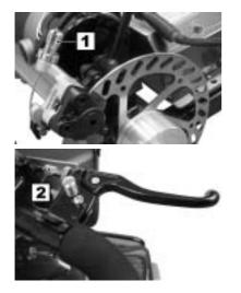
Handbrake adjustment takes place using the set screws on the caliper (1) and on the handle (2).
