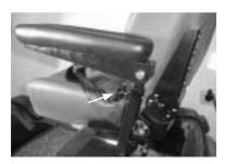
• Loosen the knob underneath the armrest, and pull the armrest up and out.
