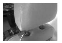
• Press and hold the release button indicated by the arrow and pull the headrest up and off.
