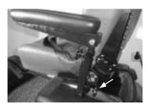
• Loosen the knob underneath the seat and remove the armrest supports by pulling them outwards.
